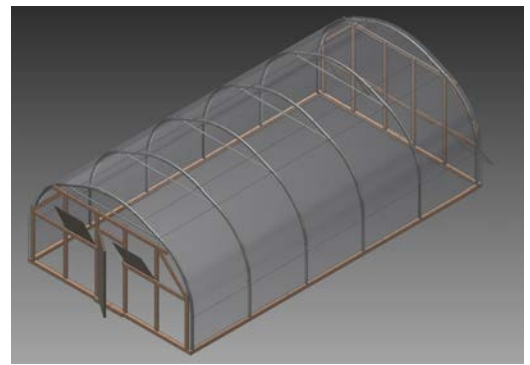
CAD image of hoop-house style mobile greenhouse
