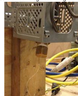
Extrusion of plastic filament from “Unprinter”
