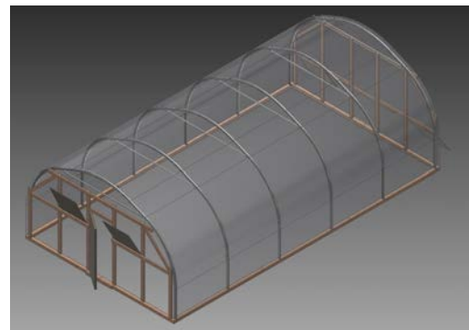
CAD image of hoop-house style mobile greenhouse
